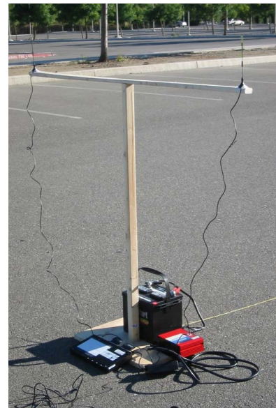
Figure 1: Photograph of one access point in our experimental setup. It includes an access point, two antennas, one inverter, one car battery and a custom-built wooden stand for the antennas.
