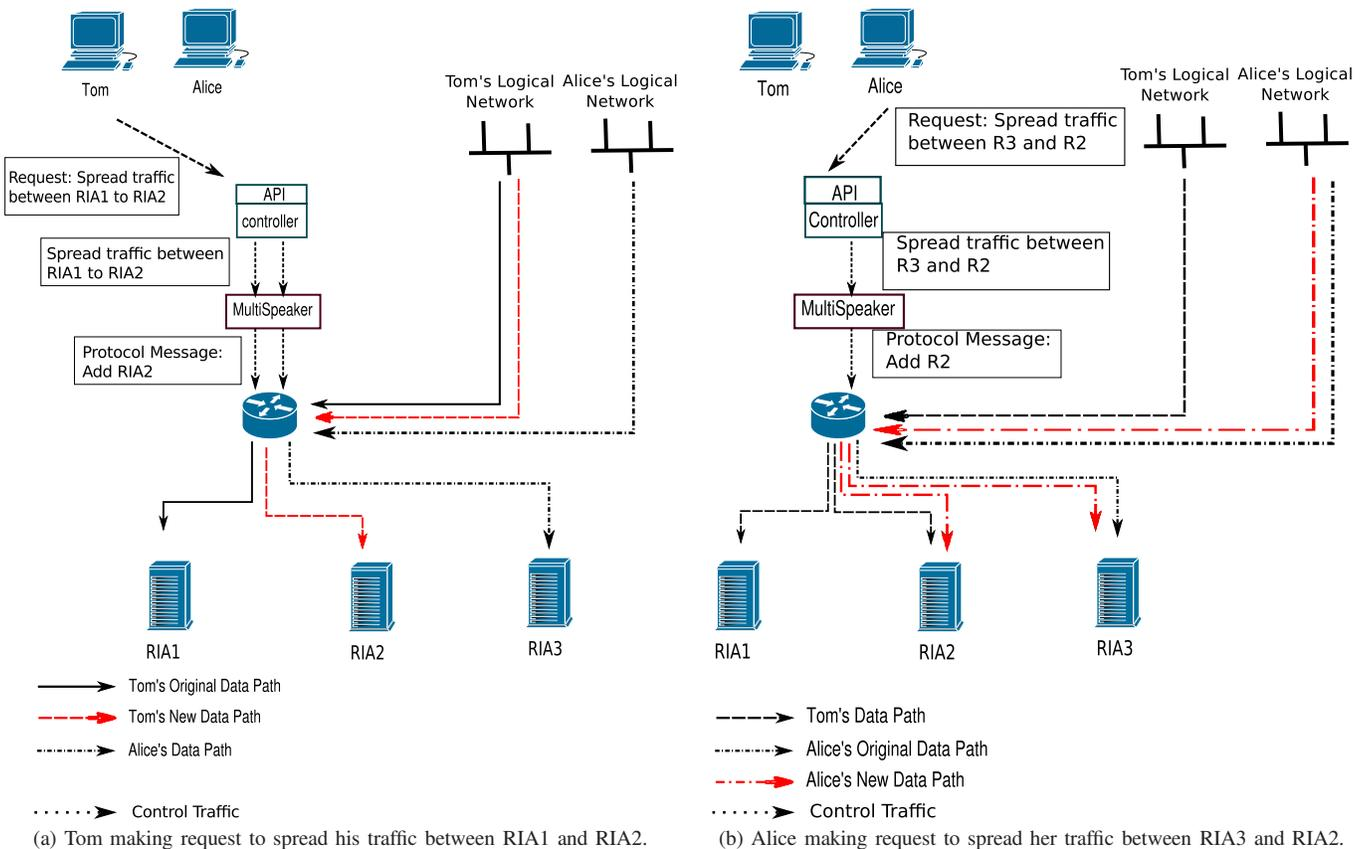
Fig. 3: Example of load balancing using RaaS.
