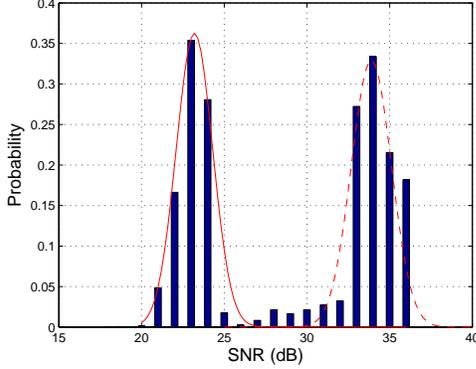
Fig. 5. Example of indoor SNR PDF: the plot shows the distribution of 123,744 frames received by a laptop in 52 minutes.
