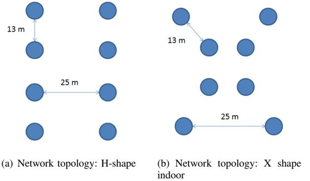
Fig. 16. Flow-level Contention Network Topologies
