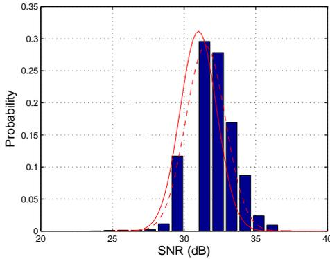
Fig. 6. Example of outdoor SNR PDF: the plot shows the distribution of 135,295 frames received by a laptop in 52 minutes.
