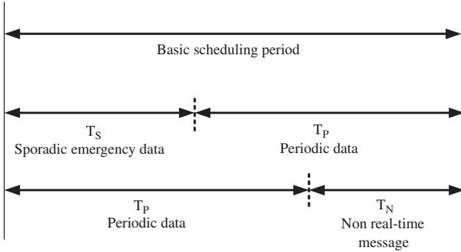
Fig. 3. Configuration of phase in a scheduling period.
