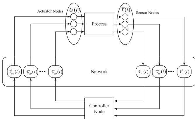
Fig. 1. Networked control loops with sensors and actuators.
