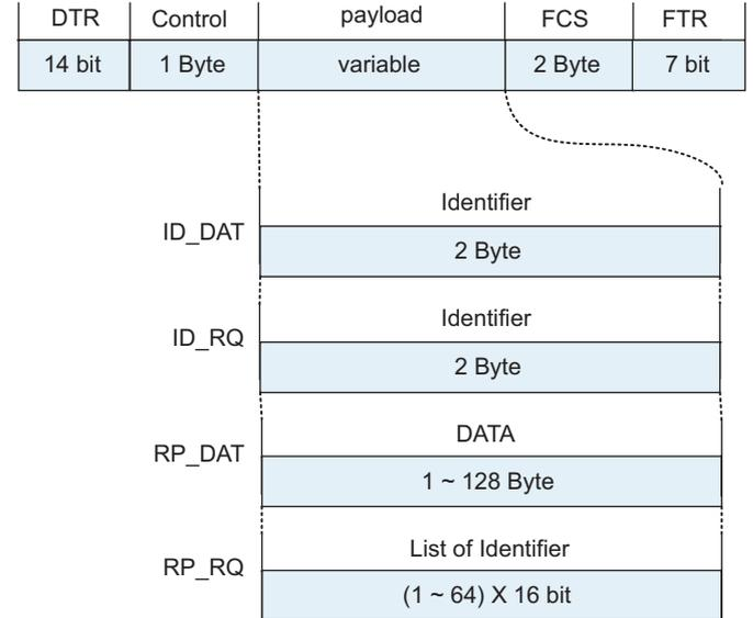
Fig. 6. Frame format of FIP.
