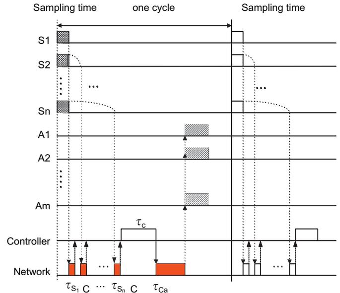
Fig. 2. Timing diagram of signals in the NCS.
