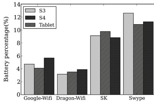
**Fig. 6.** Battery level consumption for phone and tablet.
