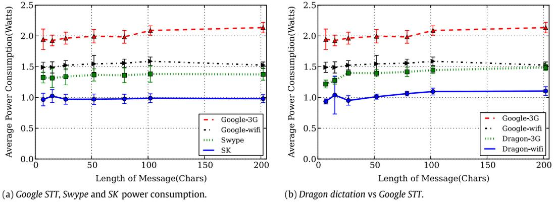
Fig. 2. Power consumption comparison of input modalities.
