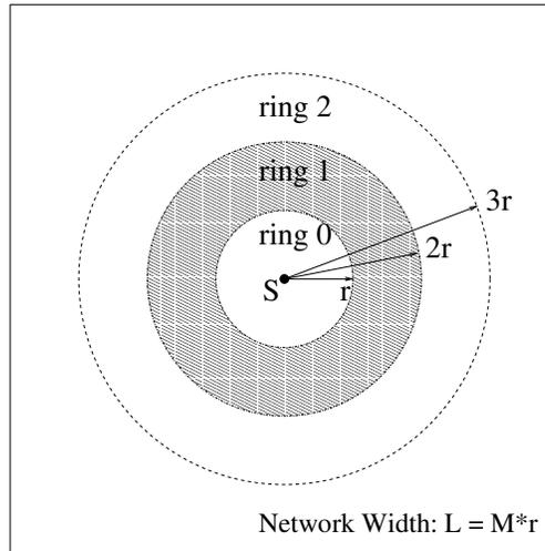
Fig. 1. The existence of “energy hole” around the sink node
