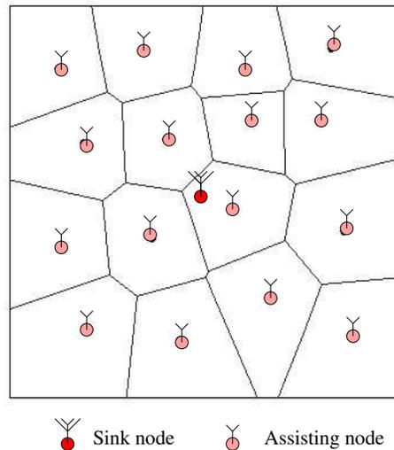
Fig. 6. Voronoi diagram due to deviated assisting nodes
