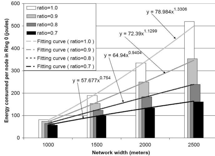
Fig. 11. Different compression ratios with different network sizes
