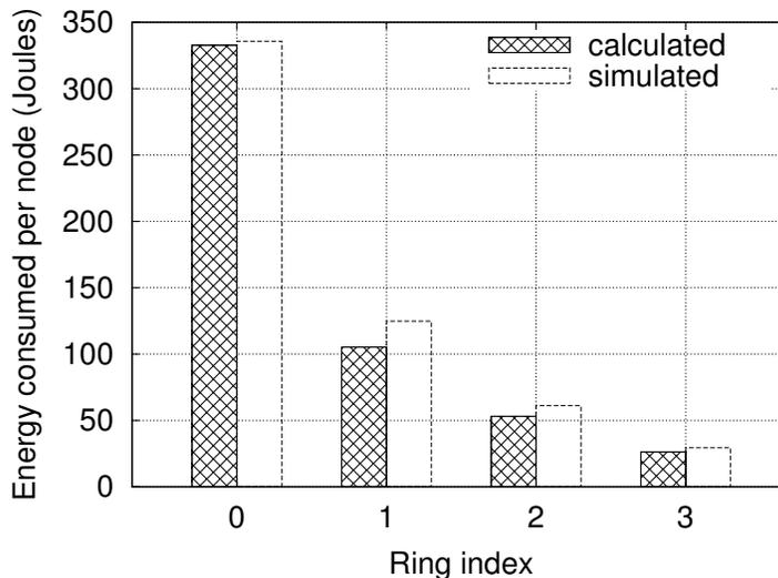
Fig. 3. Energy consumptions in different rings (when  $M = 8$ )
