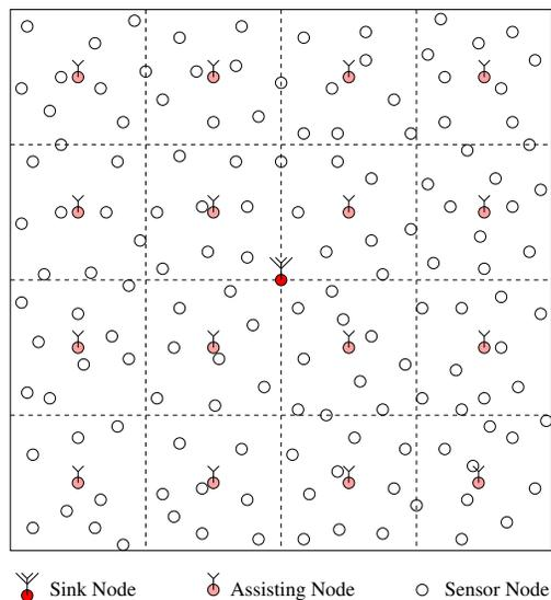
Fig. 4. An example of two-tier grid-based architecture
