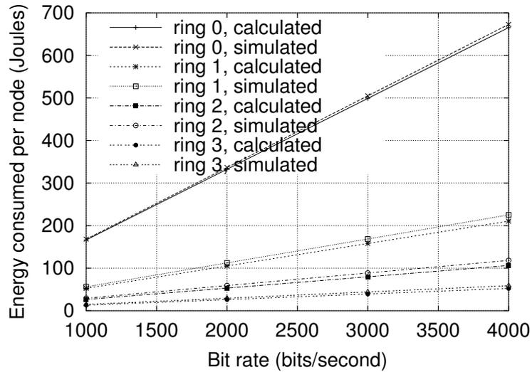
Fig. 9. Energy consumptions under different bit rates
