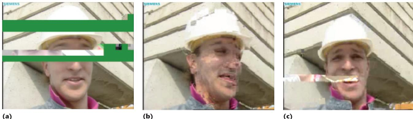
**Figure 1.** Video distortions in I, P, and B frames of a video caused by selective dropping of packets in the MAC layer (10 percent). (a) I-frame packet loss (b) P-frame packet loss, and (c) B-frame packet loss.
