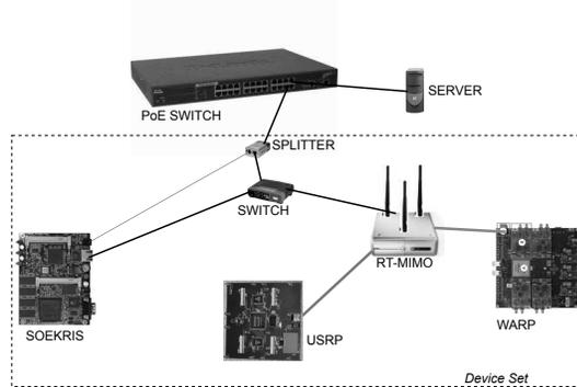
**Figure 16:** The hardware connectivity in our testbed. Each node is represented by a device set of locally interconnected platforms. The device set is connected through a PoE splitter with the other sets.
