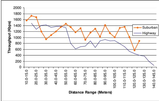
Figure 1. TCP Throughputs vs. Distance
