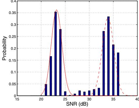
Fig. 2. Example of indoor SNR PDF: the plot shows the distribution of 123,744 frames received by a laptop in 52 minutes.
