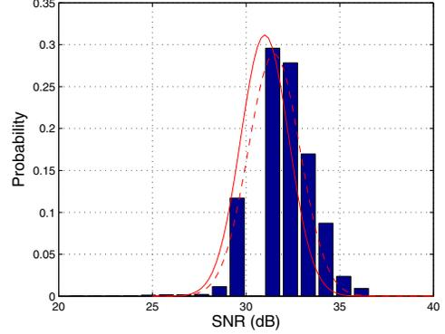
Fig. 3. Example of outdoor SNR PDF: the plot shows the distribution of 135,295 frames received by a laptop in 52 minutes.
