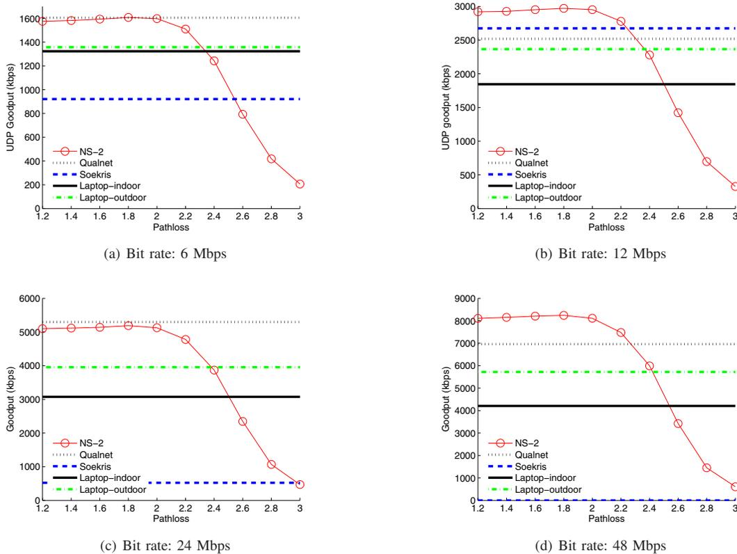
Fig. 4. Throughput varies with channel path loss at different bit rates
