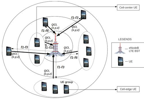
Fig. 2: Cell structure illustrating sample grouping of UEs based on geographical location and available CCs for each group, selected from range  $\{f_1, \dots, f_{10}\}$
