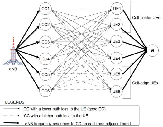
Fig. 4: Distribution of good CCs to the UEs. CC1, CC2, ... CC6 are arranged in increasing frequency
