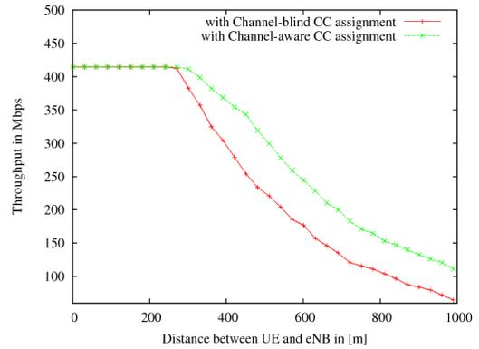
Fig. 3: Improvement of channel-aware path-loss based CC assignment over channel-blind Round-Robin CC assignment. Channel-aware scheme obtains around 57% improvement in throughput for cell-edge users with an overall improvement of 41%
