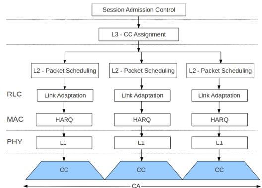
Fig. 1: Radio resource management framework of an LTE-A system
