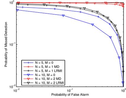
Fig. 7. Complementary ROC for primary user detection with 20% malicious nodes and  $V = 40$  m/s.
