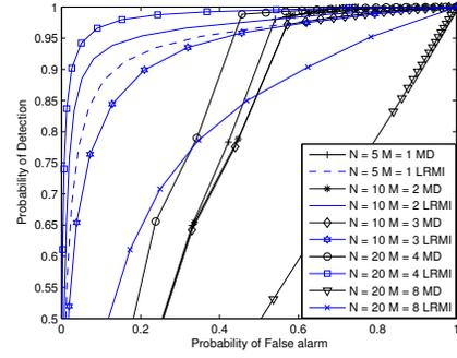
Fig. 2. Impact of secondary users - ROC for malicious user detection at  $V = 20m/s$
