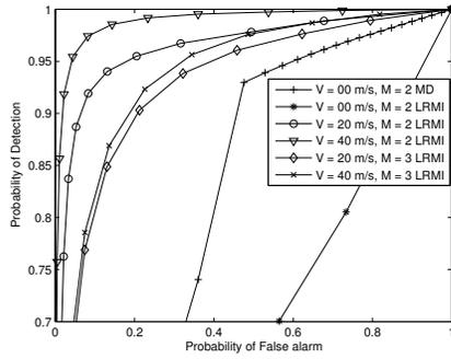
Fig. 4. Impact of velocity - ROC for malicious user detection with secondary users  $N = 10$ .
