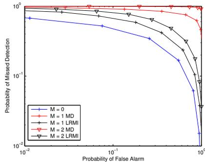
Fig. 6. Complementary ROC for primary user detection with  $N = 10$ ,  $V = 20$  m/s.
