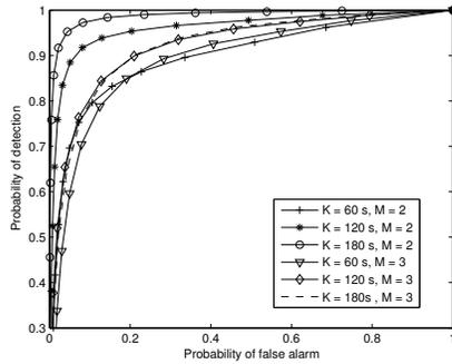
Fig. 5. Impact of LR sensing - ROC for malicious user detection.  $N = 10$ ,  $L = 9$ ,  $V = 20$  m/s
