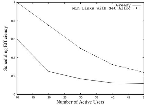
Fig. 1. Performance of ILP and Min Links with Set Allocation (1 antenna)
