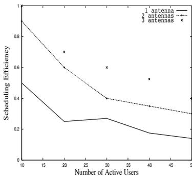
Fig. 3. “Min Links” algorithm: Number of scheduled UEs vs. number of active UEs with increasing antennas
