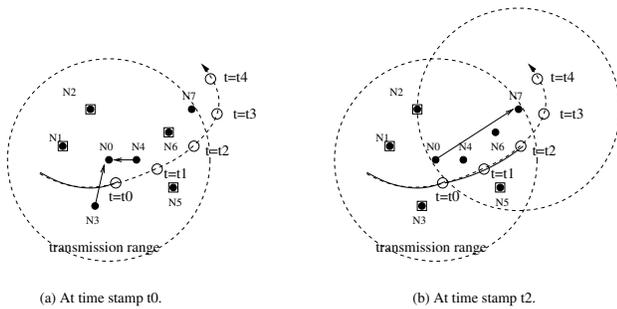
Fig. 7. Illustration of data collection along with the patrolling.
