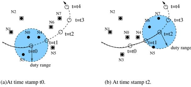
Fig. 3. The positions of the imaginary patroller at different times. Also shown are the sensors that are awake at time stamps  $t_0$  and  $t_2$ .
