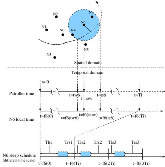
Fig. 5. An example of the sleep schedule calculation conducted at a sensor node, which is node N6 in Figure 4.
