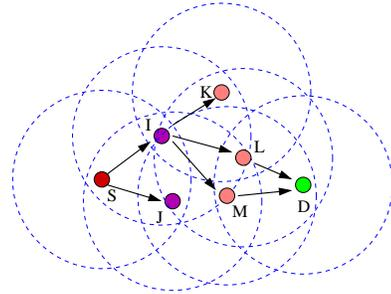
Fig. 1. “Next-hop racing”: A scenario using uniformly distributed rebroadcast delay in the flooding based route discovery process
