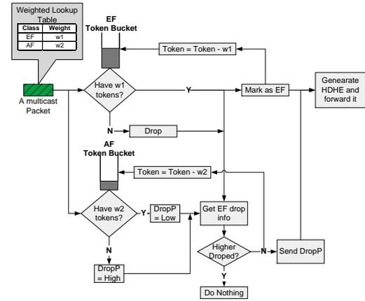
Fig. 7. Token Bucket Marking Implementation at the Edge Routers.
