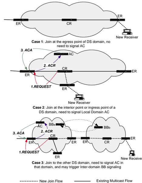
Fig. 4. Three cases of joining multicast tree in a DiffServ domain.
