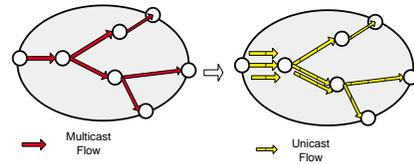
Fig. 2. Counting a multicast flow as multiple unicast flows.
