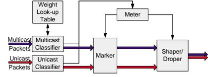
Fig. 5. Logical View of Traffic Conditioner with WTC Component.
