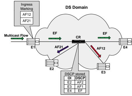
Fig. 3. Heterogeneous DSCP Encapsulation (OI: Outgoing Interface).
