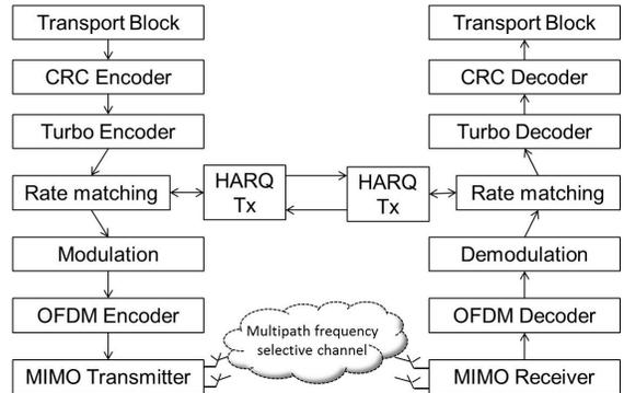
Fig. 1. Block Diagram of Link level LTE Simulator
