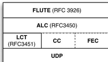
Fig. 1. Protocol stack of application layer for LTE eMBMS traffic
