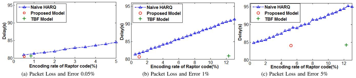
Fig. 15. Improvements in transmission delay using our model as compared to naive scheme and TBF. The input file size was fixed at 10,000 packets. The HARQ parameter (max HARQ retransmissions) for Our approach and TBF was determined by the models and kept at 3 for Naive scheme.
