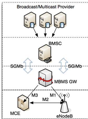
Fig. 2. Architecture of eMBMS Service
