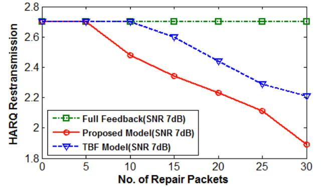
Fig. 11. Plot of average number of retransmissions with number of repair packets at 7 db, 100 source packets
