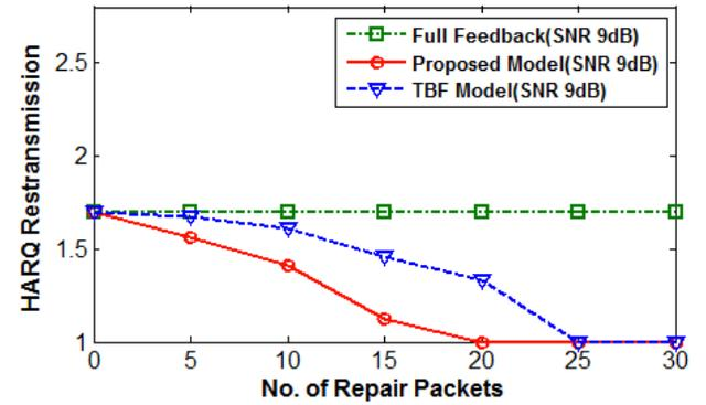
Fig. 12. Plot of average number of retransmissions with number of repair packets at 9 db, 100 source packets
