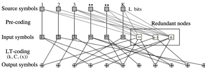
Fig. 4. Input symbols are created through Pre-coding with Source symbols, which create input symbols including redundant symbols. An appropriate LT-code make output symbols to be delivered to the receivers [13]
