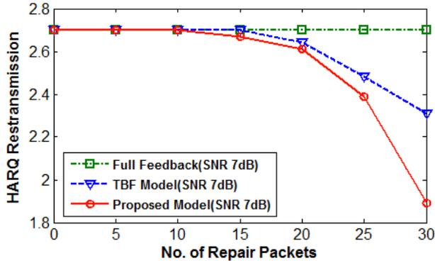
Fig. 13. Plot of average number of retransmissions with number of repair packets at 7 db, 200 source packets
