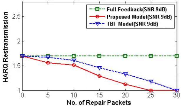
Fig. 14. Plot of average number of retransmissions with number of repair packets at 9 db, 200 source packets
