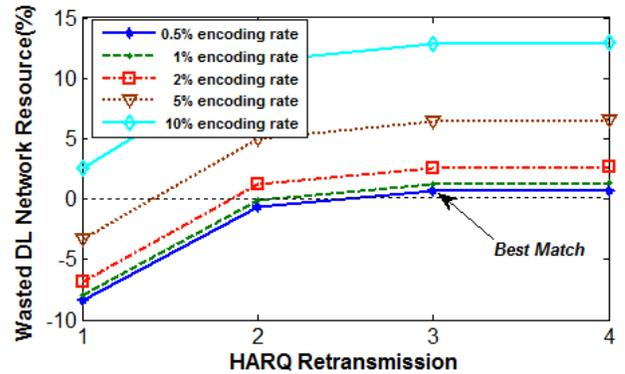
Fig. 8. Wasted DL Network resource at 0.3 loss rate
