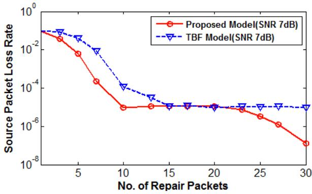
Fig. 9. Plot of source packet loss rate with number of repair packets at 7 dB
