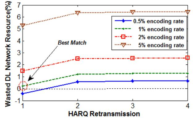
Fig. 7. Wasted DL Network resource at 0.1 loss rate
