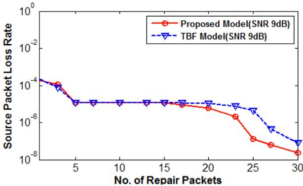
Fig. 10. Plot of source packet loss rate with number of repair packets at 9 dB
